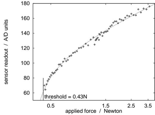
Fig. 7: **Typical trace of sensor readout vs. applied force:** The force sensitivity of the sensor is limited by a threshold that depends on the size of the gap between the foil and electrodes when no force is applied.
