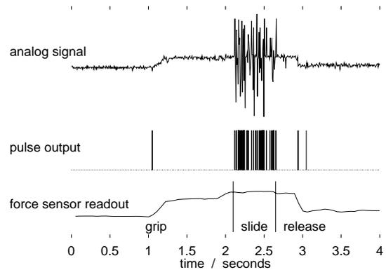
Fig. 8: **Slippage measurement during a sliding movement:** The robot arm pushes the fingertip onto a flat surface, slides, and then releases the grip. The edge detector warns if the analog slippage signal rises above a predefined threshold. Due to the low sampling rate, not all spikes are visible in the analog signal plot.
