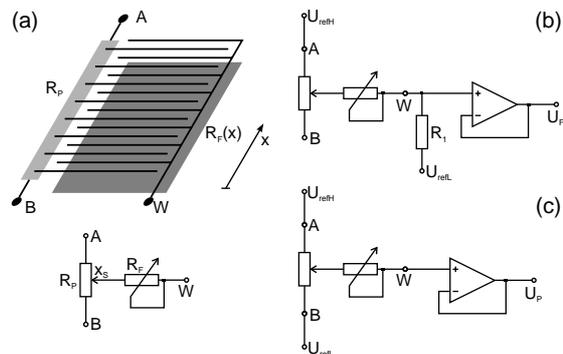
Fig. 2: **Principle of FPSR with amplifier circuitry:** The sensor consists of a set of interleaved electrodes (a) covered with force sensitive foil. The electrodes divide the foil into several fields (typically 10 to 20) that can be used for position sensing along one direction by applying reference voltages to A and B (c). Integral force sensing can be achieved with the circuit (b). To perform both measurements with one circuit, two switches are needed.
