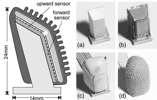
Fig. 5: **Mechanical design of the fingertip:** The photos show intermediate phases in the construction of a tip.
