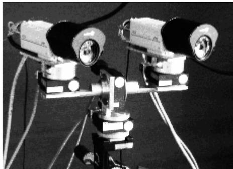
Figure 15: The active stereo camera head offers 4DOF for head gaze control (pan, tilt, and vergence) as well as 3DOF in both motor lens system (focus, aperture, zoom).
