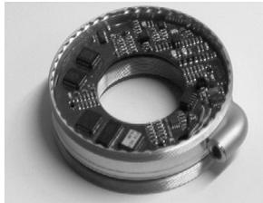
Figure 9: The DLR wrist sensor for sensing all six force and torque components acting in the (virtual) sensor center between the upper and lower part. The on-board electronics measures, pre-filters the primary strain-gauge sensors, and computes and transmits the temperature compensated results.
