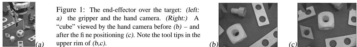
Grasping without any alignment help requires that the objects are picked with certain precision. Failures include the risk of (i) object–gripper collisions, (ii) pushing/displacing something before yaw closure, and (iii) bad object-in-gripper alignment (creating trouble for later part mating).
